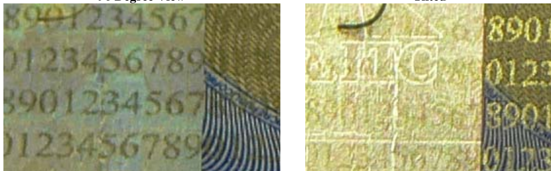
Figure 11 Angle Dependent Metallic Variable Effect Integrated into an OVD
