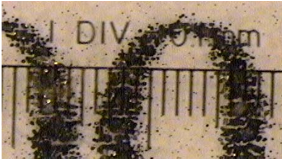
Figure 5 Image of High DPI Characters Printed on a Home Thermal Printer
