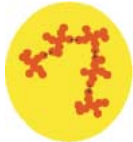
Fig. 2: A strong oxide-oxide attraction forms networks and controls the rheology.
