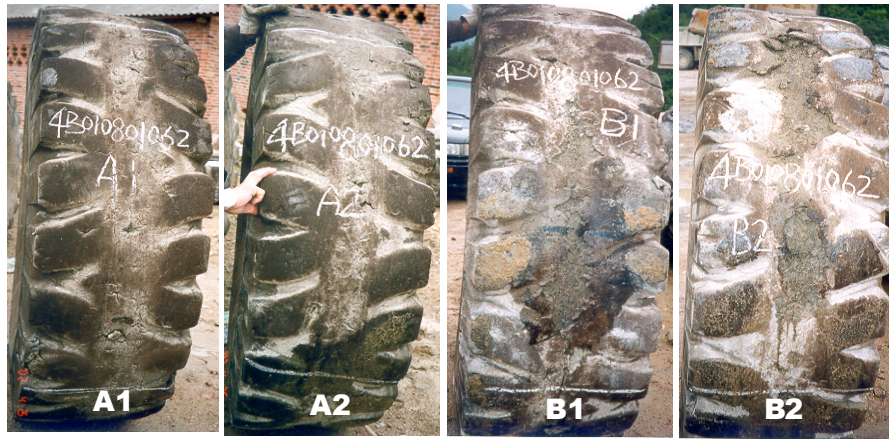
Figure 7: Photographs of tire prepared with two-section tread, showing condition of tire after off-the-road use.
