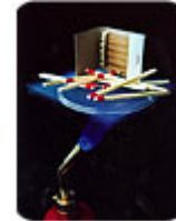
The matches resting on top of the aerogel are protected from the flame underneath. Photo courtesy of NASA/JPL-Caltech.
